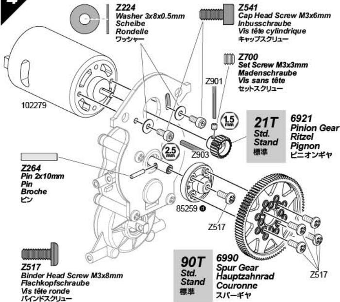
Proper Spur Gear Mesh
