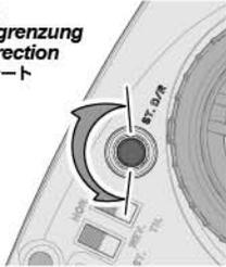
To be used to adjust steering servo throw.
