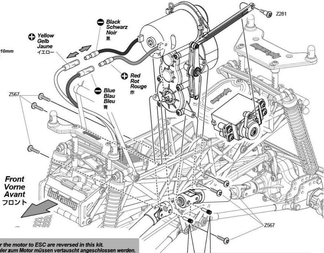
**The connections for the motor to ESC are reversed in this kit.**
